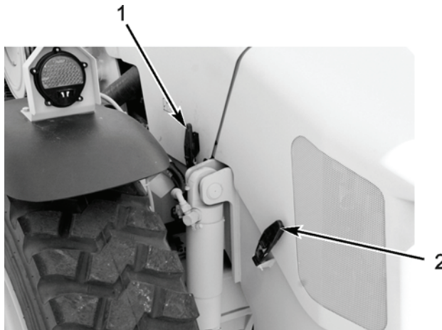
Figure 86. Opening Hood and Nosecone
